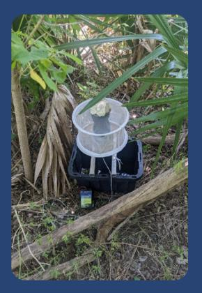
On the left, you can see a Gravid Trap, which was designed by Dr. Paul Reiter of the Centers for Disease Control, Division of Vector-Borne Disease for the selective capture of gravid Culex mosquitoes. By limiting captures to this class of females, problems associated with calculation of minimum virus infection rates were reduced.
